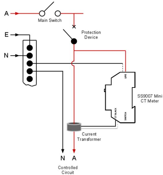
A Cable of minimum cross section 0.1mm and maximum cross section 1.5mm (stranded) or 2.5mm (solid core) may be used. The device must be connected in the correct polarity to ensure proper operation. The Live terminal, Neutral terminal, two Current Transformer (CT) terminals (“CT BLACK” and “CT WHITE”), and two SWITCH terminals are marked on the side of the device enclosure.
